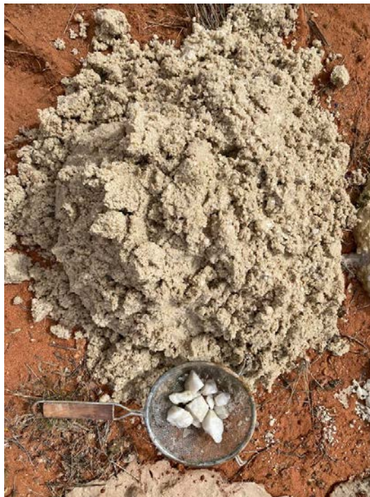
Figure 5. Sand and Silcrete at 85m from LWP002
