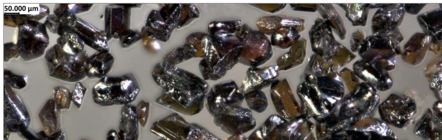
Figure 8: Photomicrograph of high purity rutile product 97.2% TiO 2
