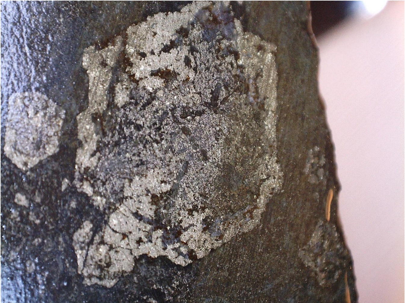
Figure 5. Recrystallised metamorphic hexagonal pyrrhotite-pyrite porphyroblast within chloritised interval in Diamond Drill Hole 97DGD006 at 200.20m. The drill core is NQ2 size, diameter 50.6mm, cut in half, the field of view is 18mm. It is estimated that the pyrite rimmed pyrrhotite shown represents less than 2% of the mineralised section 200.20 – 200.40m.
