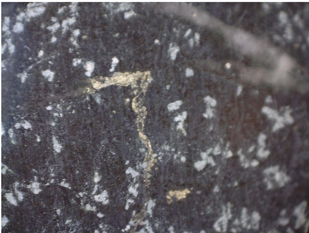
Figure 3. View of sulphide blebs within pyroxene poikilitic gabbro in Diamond Drill hole 97DGD002 at 200.00m. The drill core is NQ2 size, diameter 50.6mm, cut in half, the field of view 18mm. It is estimated that the pyrite sulphide shown represents less than 1% of the mineralised section at 200.00m
