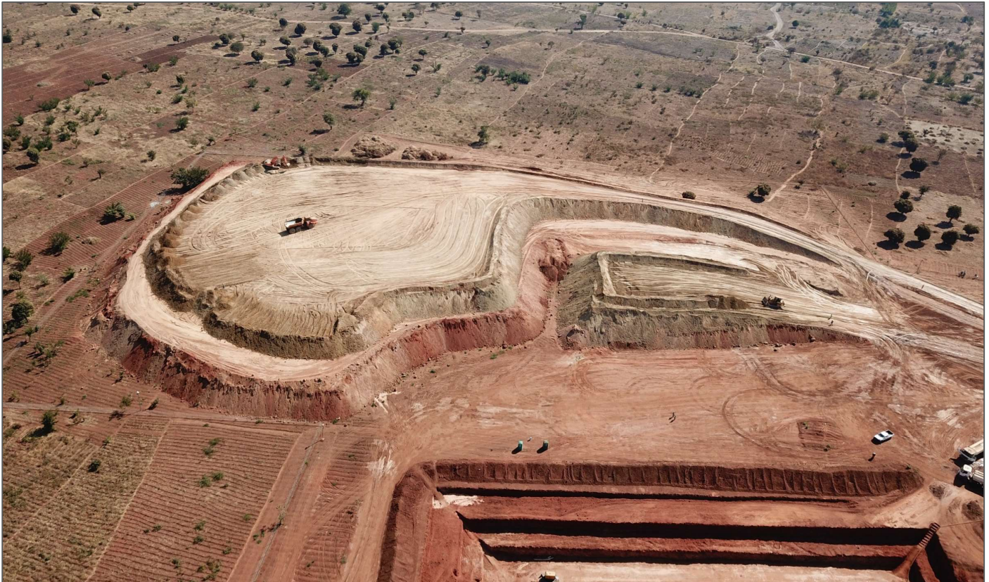
Figure 5: Dry mining plant feed stockpiled without any crushing or grinding
