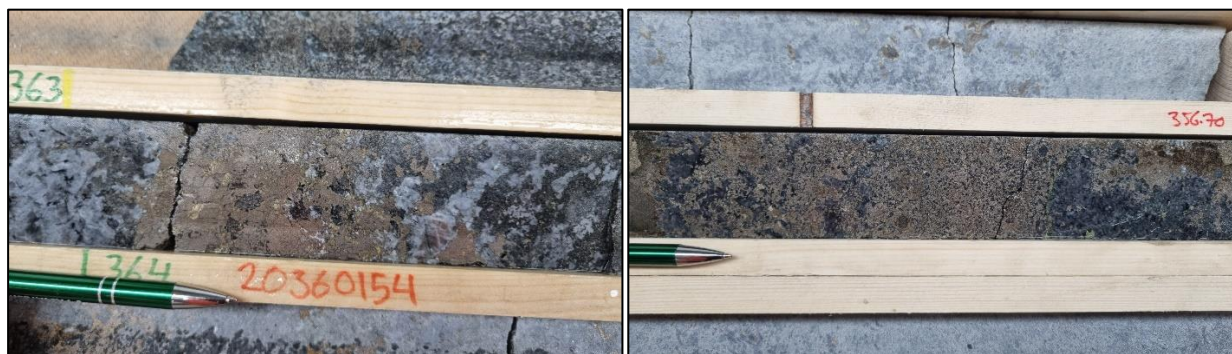
Plate 1 (Left): Massive and blebby pyrrhotite-pentlandite-chalcopyrite hosted by coarse grained gabbro from a 1.48 m sample that returned 1.8% Ni, 0.2% Cu, 0.08% Co from 273.22 m, KUSK0015 (RTX drilling). Plate 2 (Right): Massive pyrrhotite-pentlandite-chalcopyrite hosted by medium grained pyroxenite from a 0.54 m sample that returned 3.7% Ni, 0.20% Cu, 0.15% Co from 361.0 m, KUSK0015 (RTX drilling).
