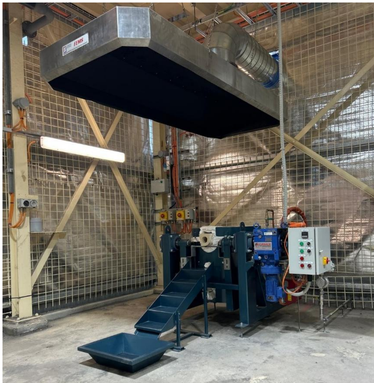
Figure 1: Smelting furnace commissioned within the Blackjack gold room ahead of the first gold pour expected next week
