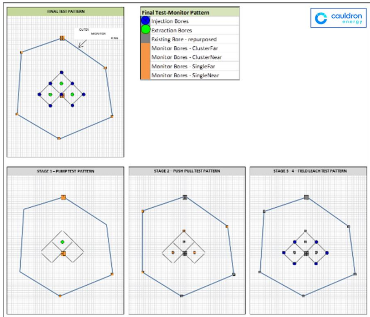
Figure 26: Design of the Proposed Field Leach Trials
