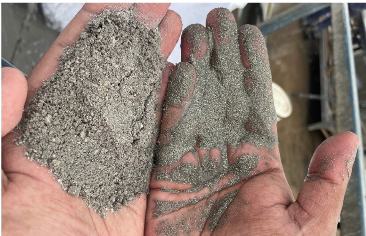
Figure 5 – Feed ore milled to <4 mm on left hand, and gravity concentrate on right hand.
