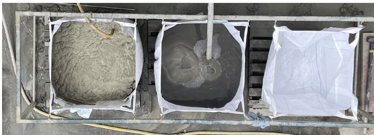
Figure 3 – Collection of concentrate into 1 tonne bulka bags with float concentrate on the left, and gravity concentrate in the centre.
