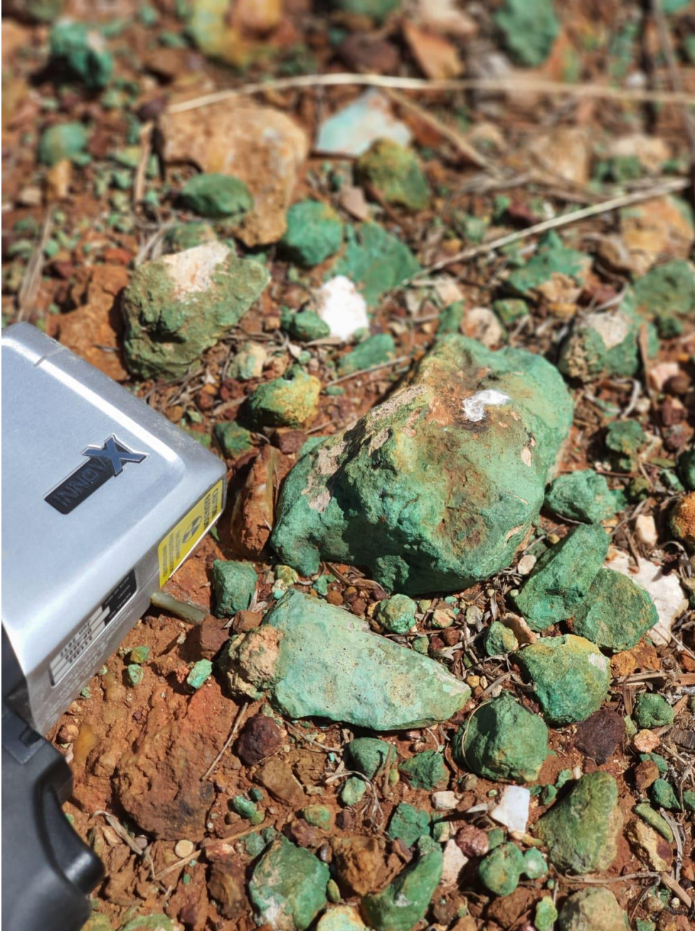
Figure 4 Crosswinds Copper Prospect - Malachite (copper carbonate) mineralisation exposed at surface
