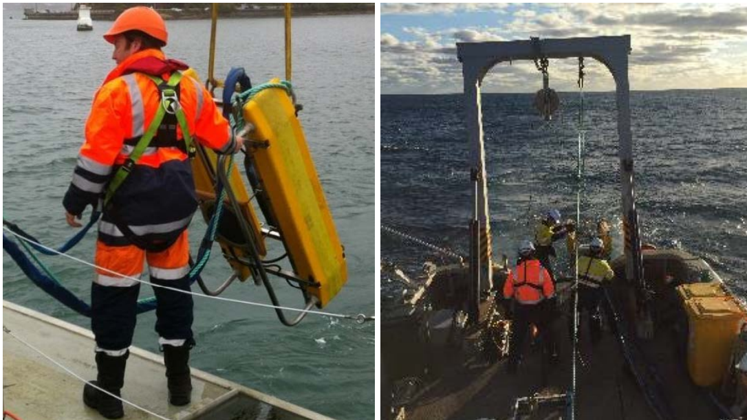
Catamaran mounted sub-bottom profiling equipment being deployed from survey vessel
