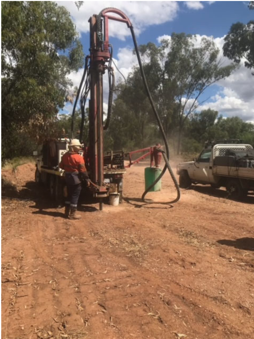
Figure 2: Aircore Drilling Currently Underway at Javelin's Husky Project, NSW (Photograph courtesy of Javelin's Consultant's Rangott Mineral Exploration Pty Ltd)
