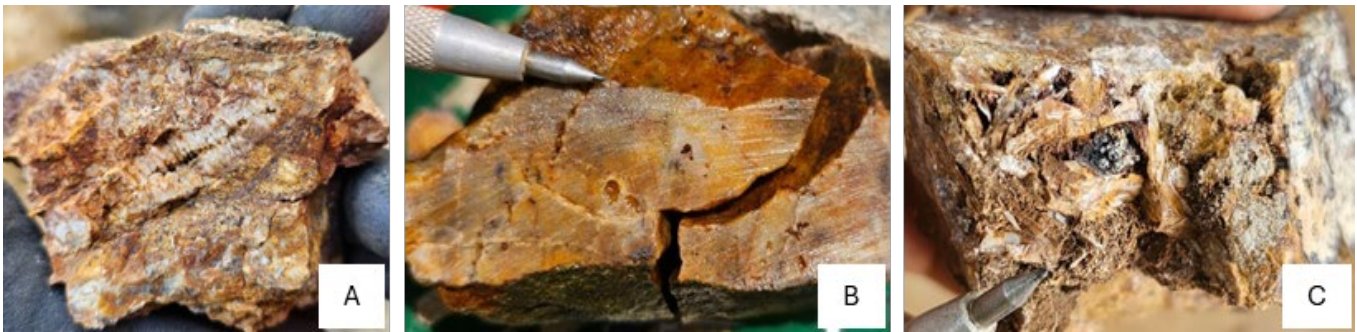
Hand specimens taken from the Iguana prospect. A: Epithermal quartz vein, comb texture with jarosite, goethite, traces of hematite. B: Epithermal quartz vein, massive texture, traces of pyrite, goethite, and hematite. C: Epithermal quartz-barite vein with goethite, the quartz shows massive texture, while the barite shows bladed texture.
