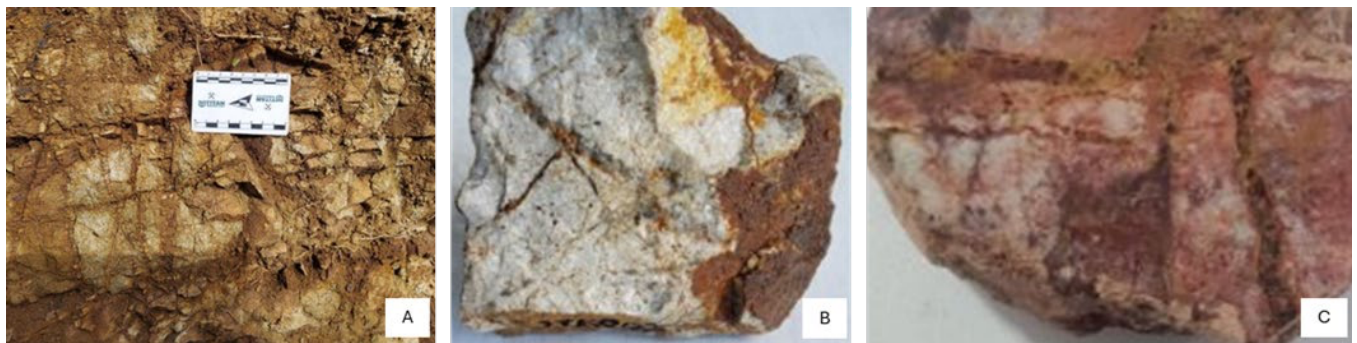
Trench and hand specimens taken from the Gisell prospect. A: Oxidised sulphide (iron oxide) veins revealed in trenching. B: A-type vein uncovered in trenching. C: Oxidised sulphide (iron oxide) veins with irregular boxworks texture.
