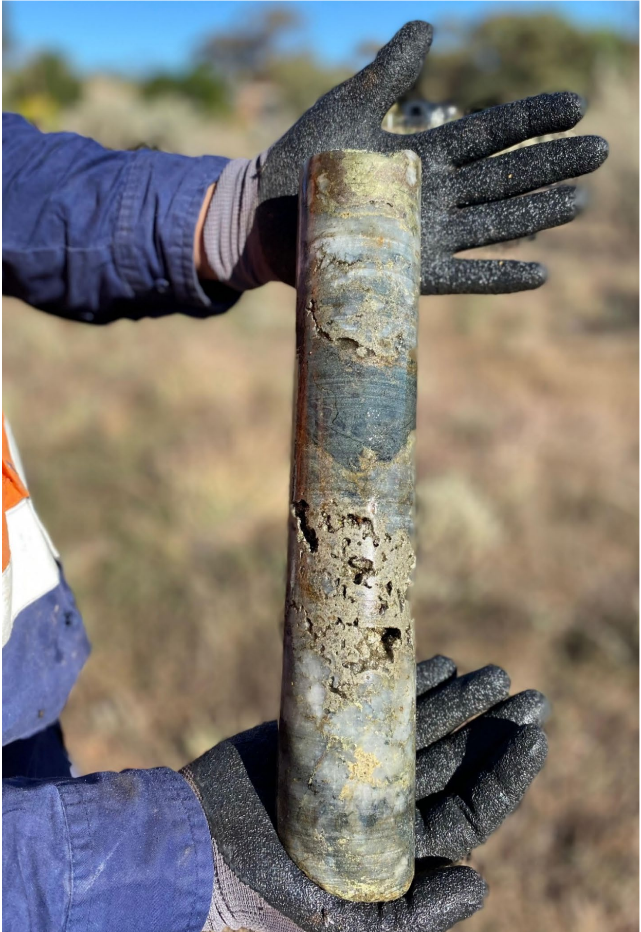
Figure 1 Diamond drill HQ core fragment, Paris Gold Project. Hole 24PRCDD096, from 154.21m to 155.98m. Chalcopyrite, pyrite, albite alteration and visible gold mineralisation. The presence of visually recorded minerals should not be interpreted as an indication of grade. Assays are imminent and will be announced as soon as available.
