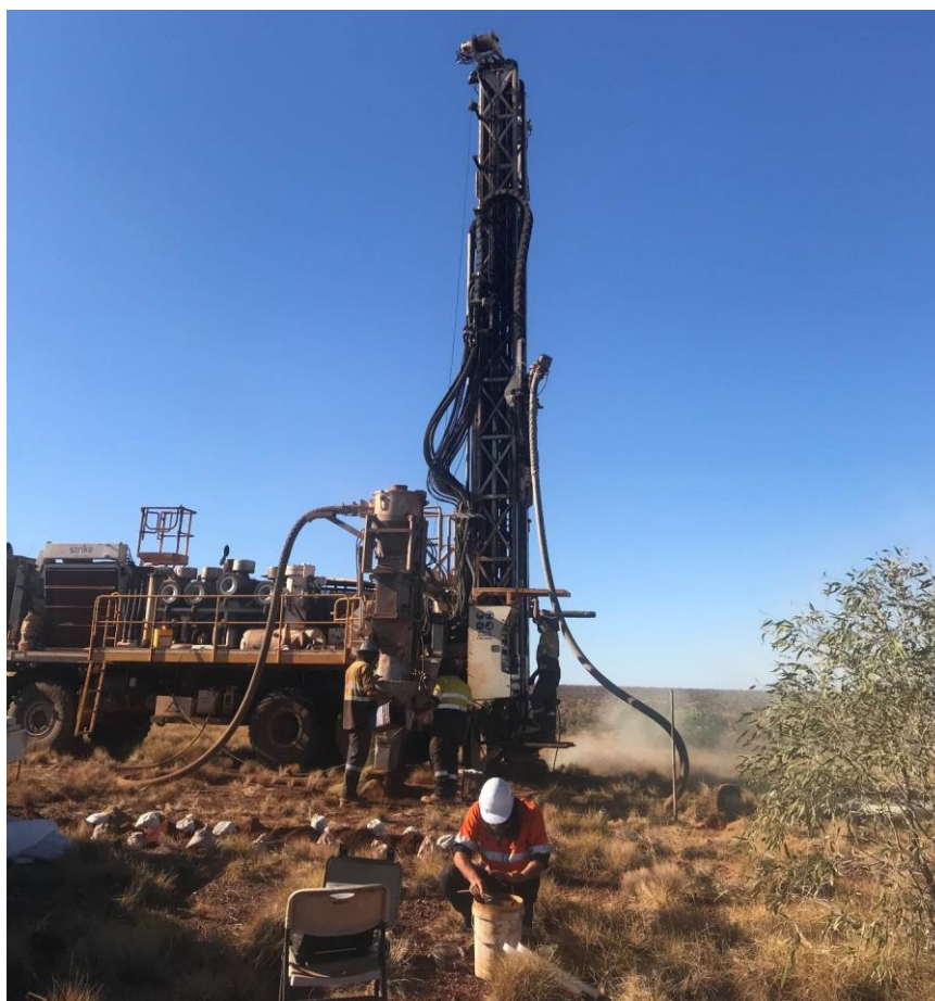
Figure 2 - RC drilling at the Lake Mackay Project, May 2019
