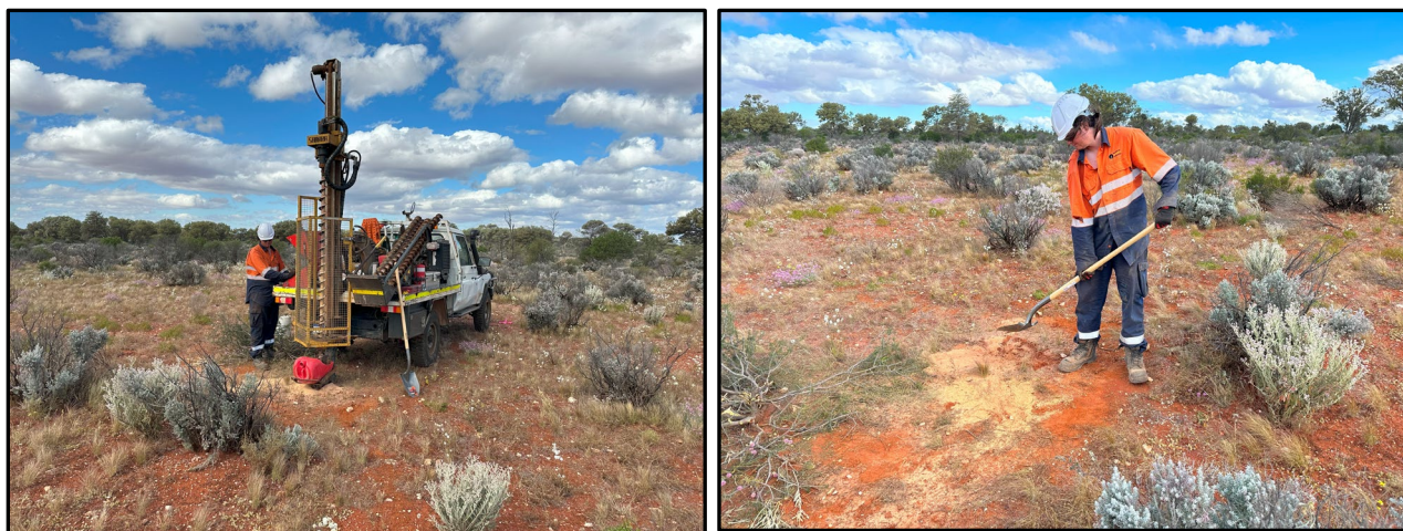
Photo 1: Mechanised augering at Pinjin East. The augering requires no clearing resulting in a minimal disturbance. All holes are backfilled on completion.
