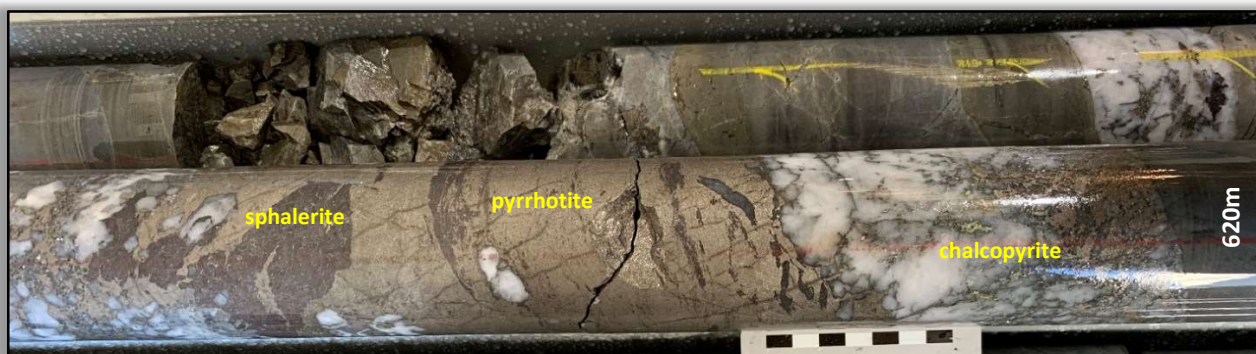
Figure 1: Core photography of massive pyrrhotite + quartz ± sphalerite ± scheelite ± cassiterite ± chalcopryrite mineralisation in TBD001, from 620m
