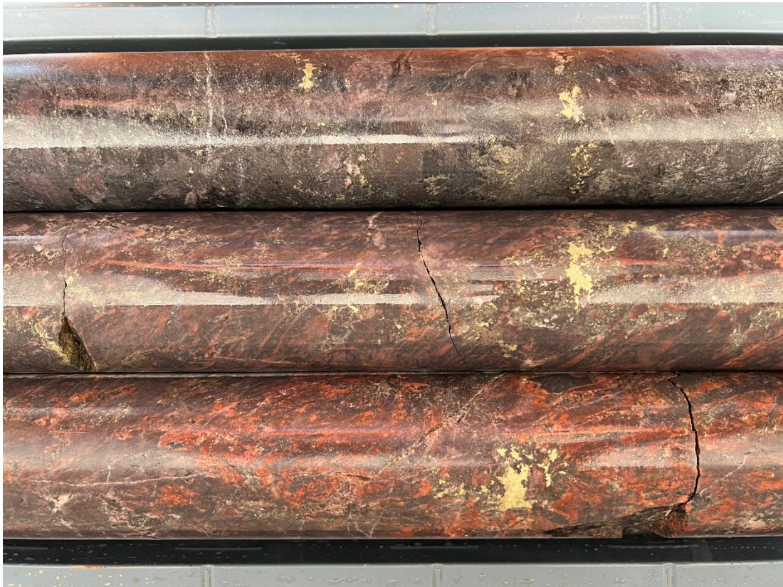
Figure 8: Examples of heavily altered volcanics with copper sulphide mineralisation from drill hole WL22DD001 (Wills target) between 575-577.7m. Copper sulphide (chalcopyrite) is yellow.
