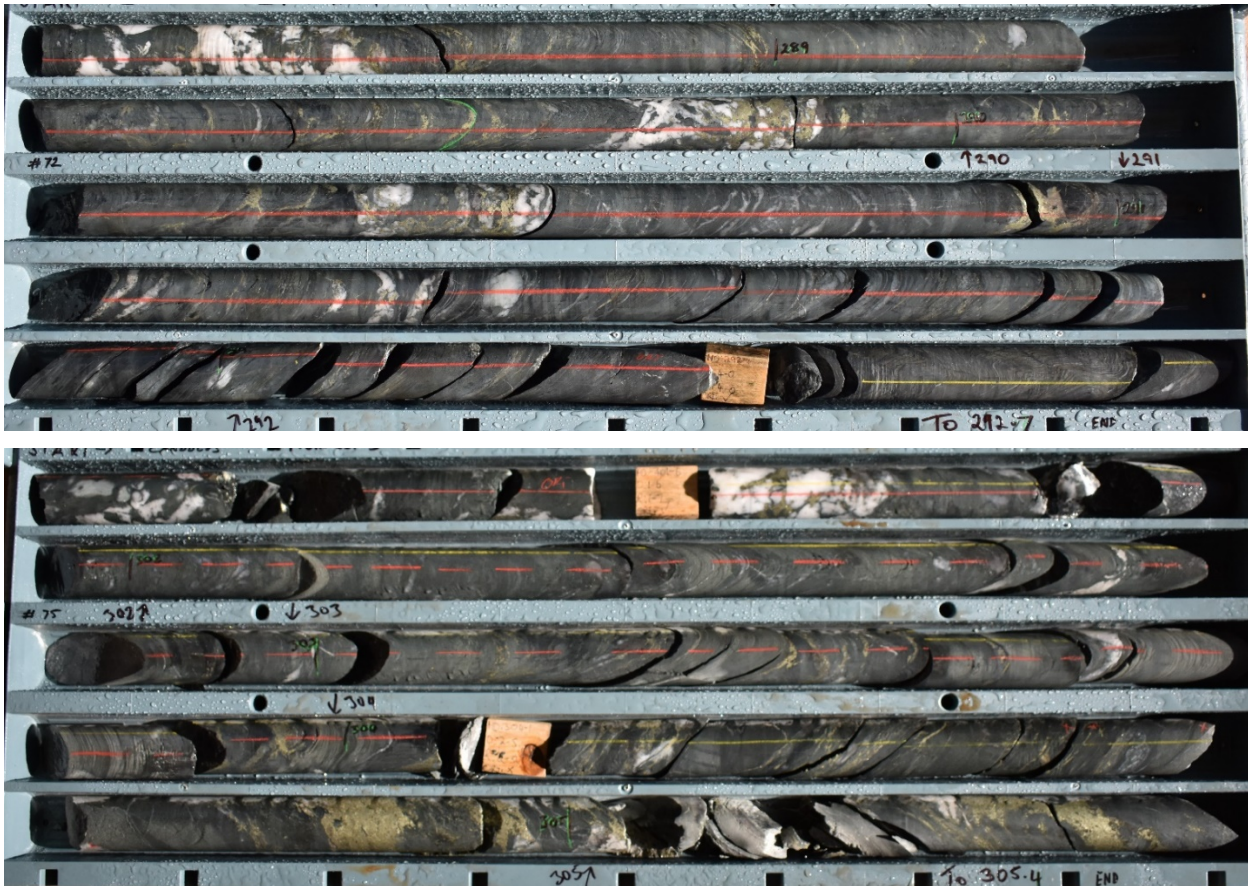
Figure 1: Stringer, vein and disseminated chalcopyrite 3 in drillhole CANDD003. The upper core tray is from 288.4m to 292.7m and the lower core tray is from 301.3m to 305.4m.
