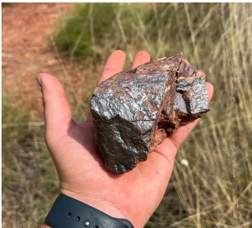
Figure 6: Oxidised Chalcocite mineralisation at BOGS1 Site
