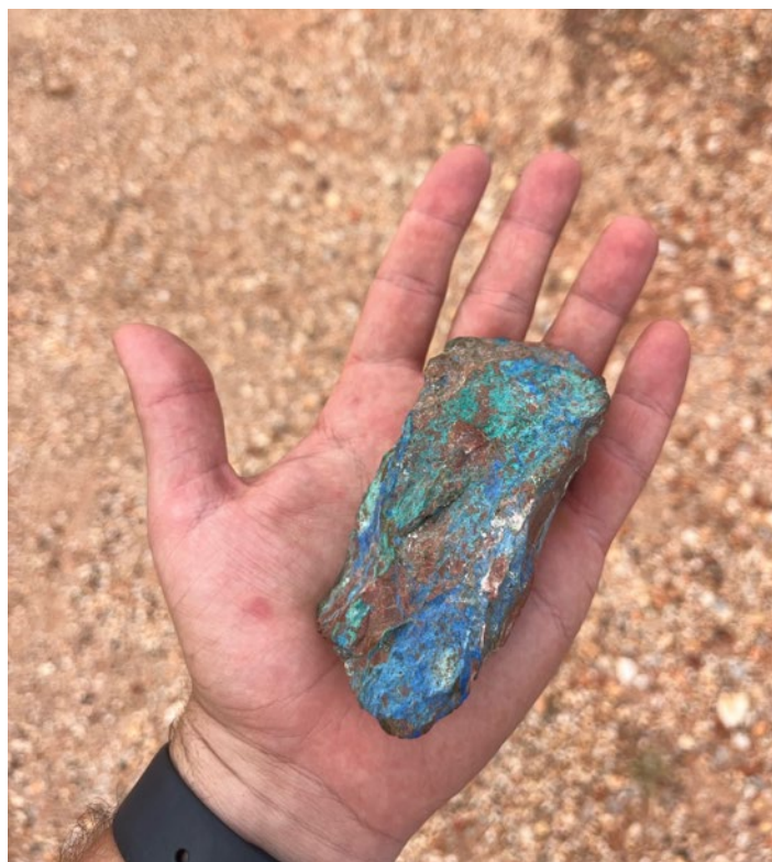
Figure 4: Disseminated azurite and malachite alteration throughout silicified sedimentary unit at BOGS3 Site
