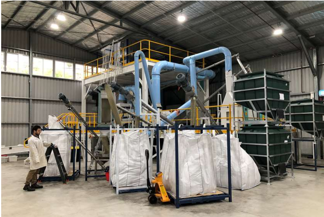
Figure 2: APH's de-hulling and sorting machine
