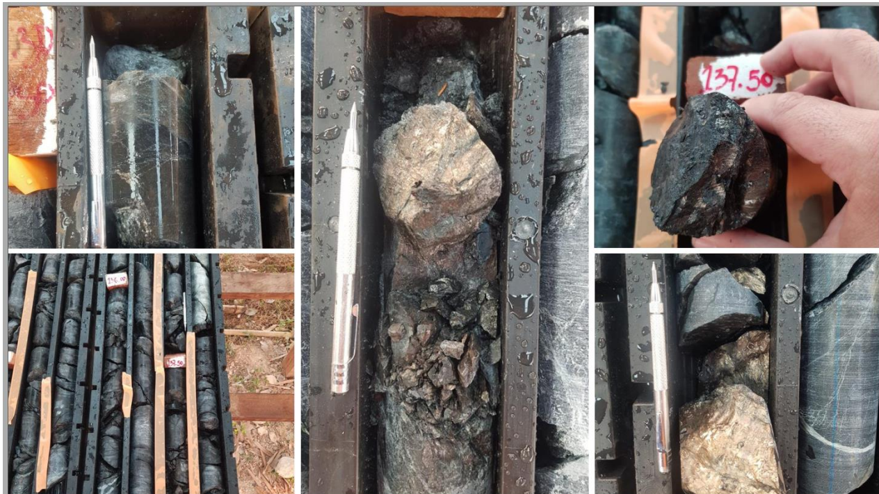
Figure 4: Massive sulphide mineralisation intersected in PLDD008. Orange tape on core trays in bottom left image denotes zones of layered sulphides.
