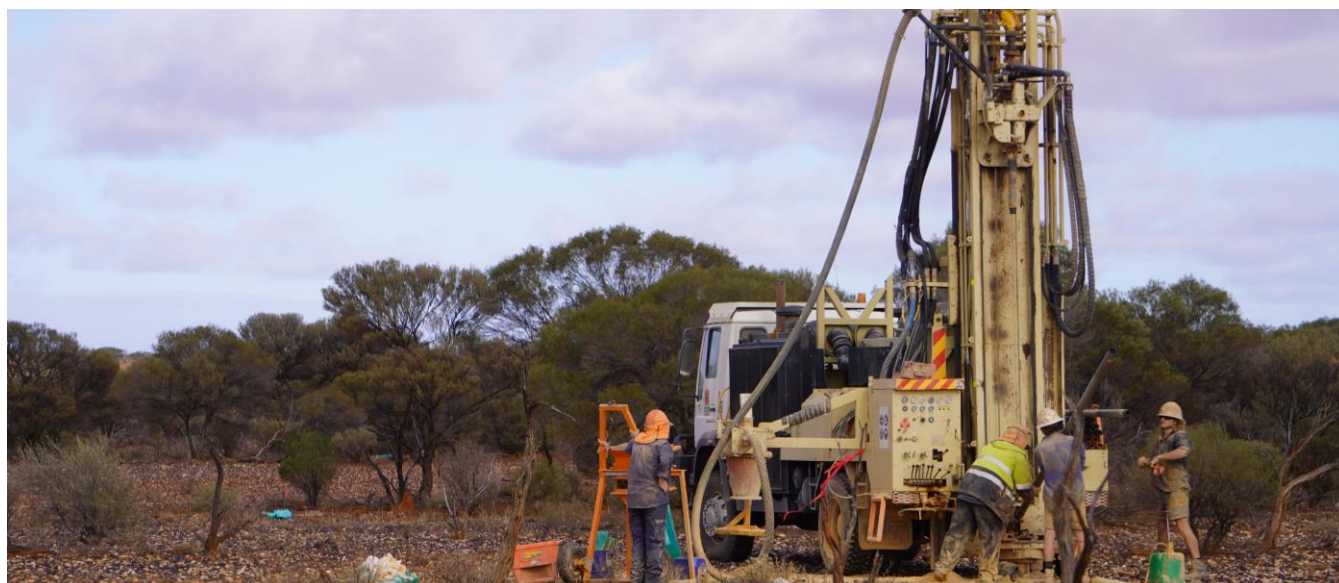
Figure 2: Reverse circulation drilling at the company's Mt Stirling Project.
