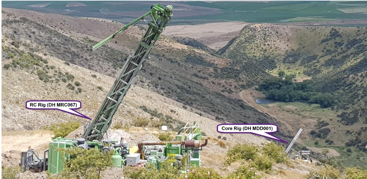
Figure 4 Come-in-Time (CIT) drilling (view NW)– RC and DD rigs drilling in tandem
