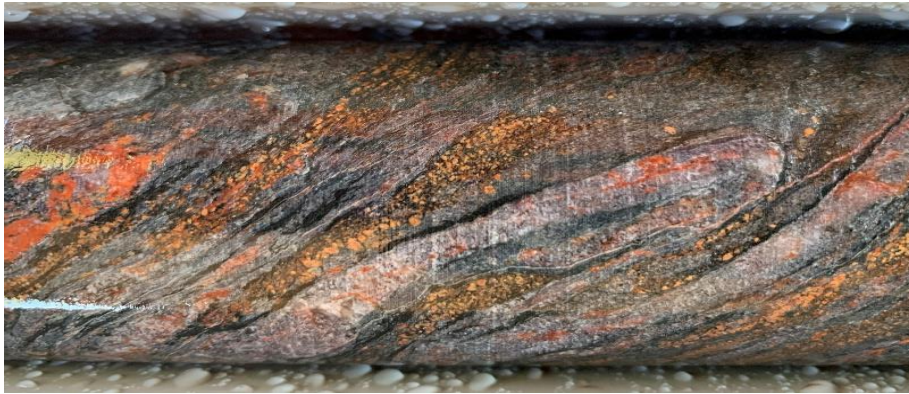
Figure 9: Ductile deformation (folding) in hematite altered biotite-rich metasediments – Hole Depth: 323.5m
