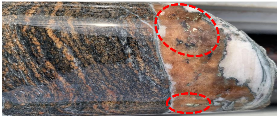
Figure 10: Pyrite-chalcopyrite (copper mineral) mineralisation within a siderite-albite vein within biotite schist – Hole Depth 497m
