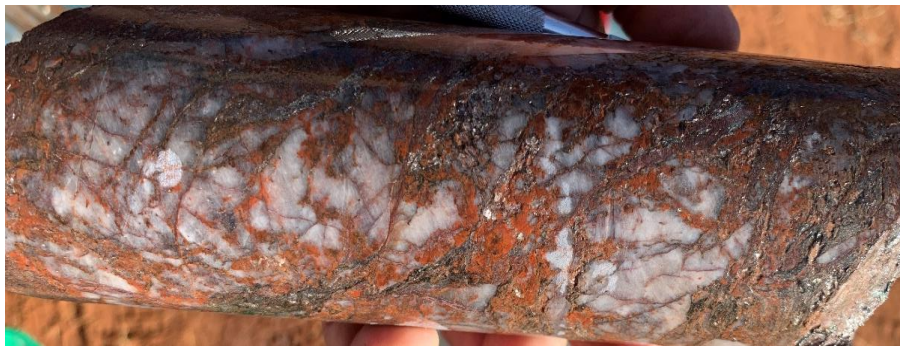
Figure 7: Hematite alteration in quartz crackle breccia – Hole Depth: 293.1m
