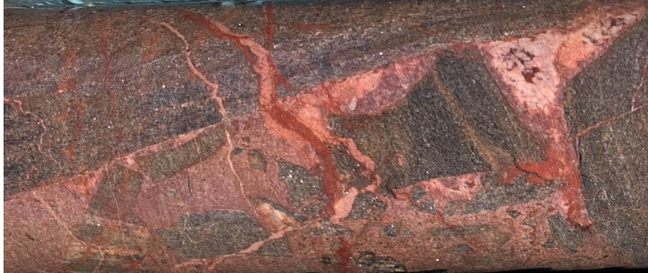
Figure 6: Crackle breccia with matrix of Qtz, Feld, Carb & Hem – Hole Depth: 277.7m
