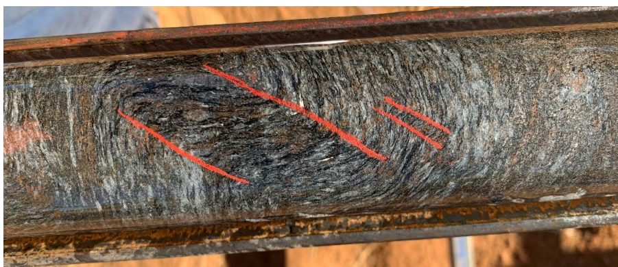
Figure 11: Hematite alteration developed within fold axes (marked in red) between 530-540m – a structural configuration observed in Tennant Creek ironstone deposits
