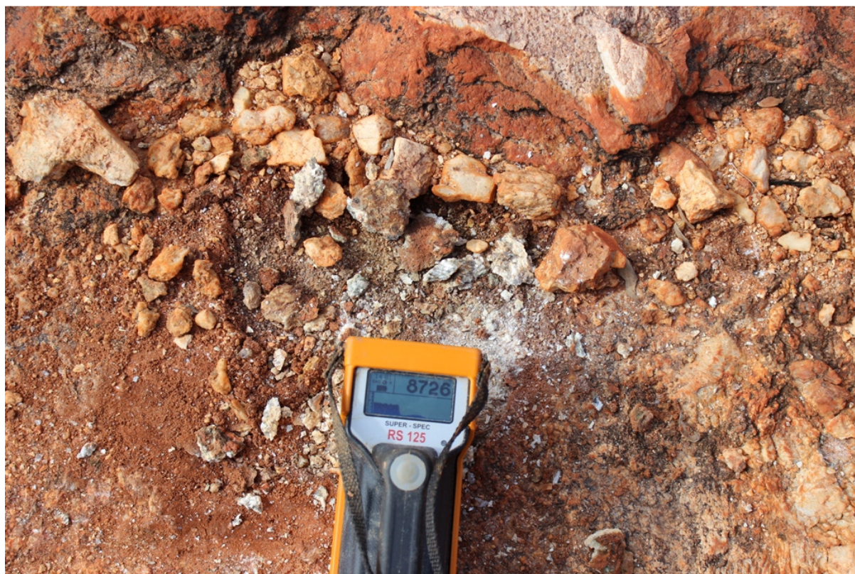
Figure 5 - Surface radiometric readings associated with hot spot within coarsely crystalline granite. Site of sample # 048348.
