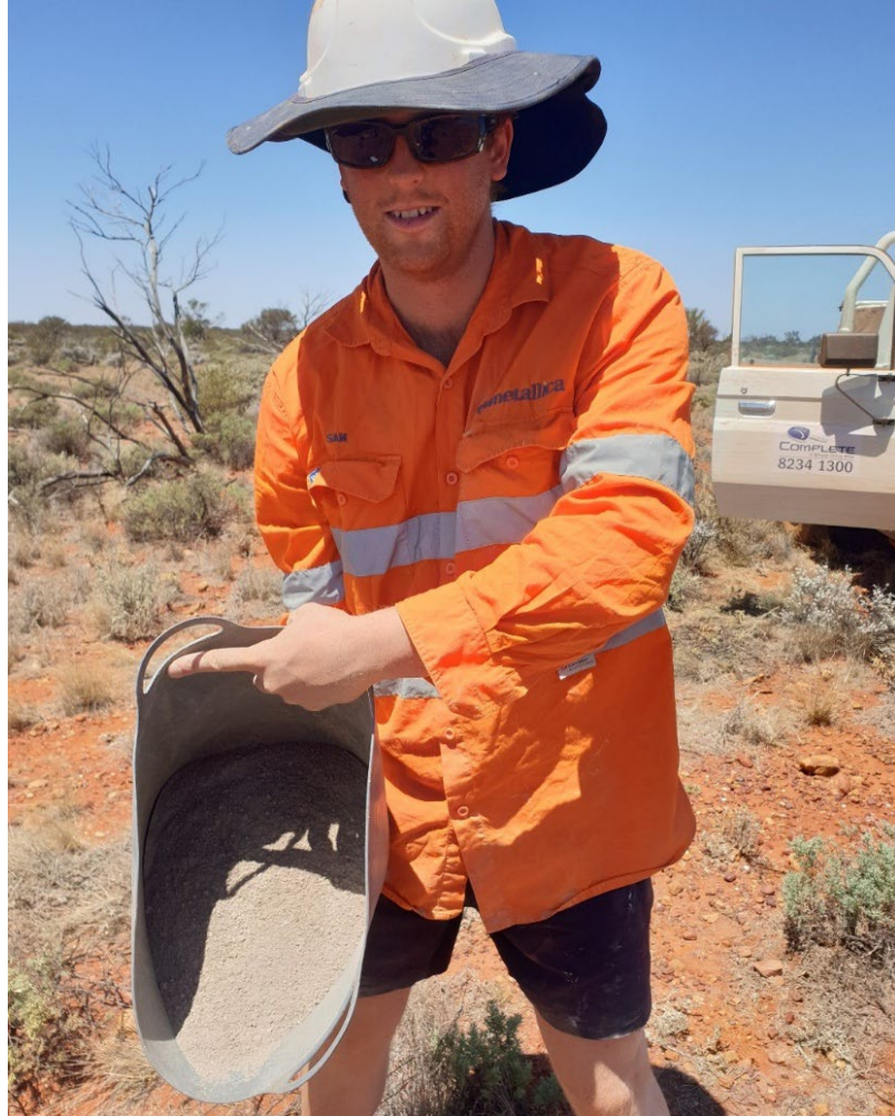
LEFT - High-grade Heavy Mineral Sand Interval - (drill hole 24RW049, 8-9m). Sands become distinctively dark grey due to high heavy mineral content. RIGHT – Panning of same interval highlights Heavy Minerals. HMC = 31.2%.
