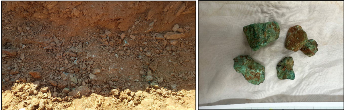
Photo 1: Copper (malachite) mineralisation in surface excavation and malachite rich chips at Browns prospect.
