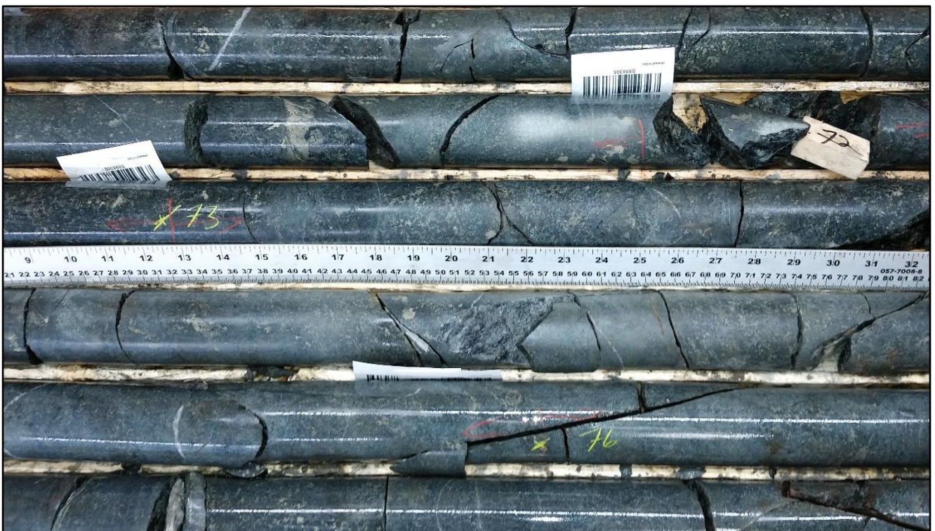
Figure 6: ZA-19-08 – gabbro with disseminated and net textured pyrrhotite-pyrite-chalcopyrite mineralisation at 71-76m downhole.
