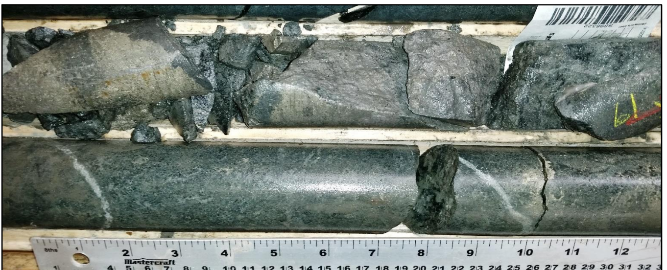
Figure 4: ZA-19-07 - semi-massive sulphide mainly pyrite with lesser pyrrhotite at 61m downhole in gabbro.
