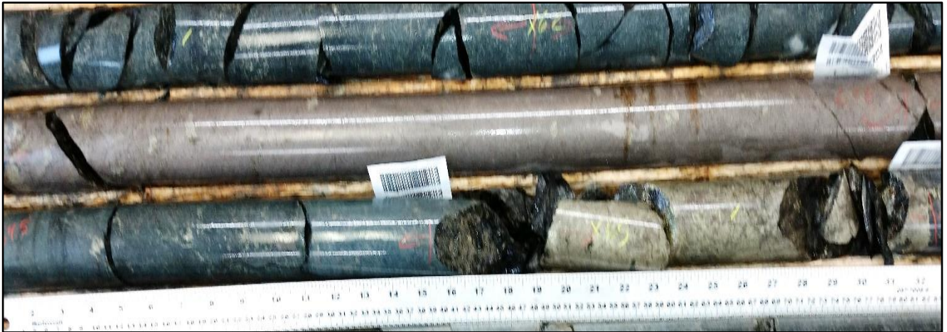
Figure 5: ZA-19-08 massive pyrrhotite with 5-10% pyrite at 63 to 64.5m downhole and 40cm semi-massive chalcopyrite with 10% pyrrhotite at 65.1m.
