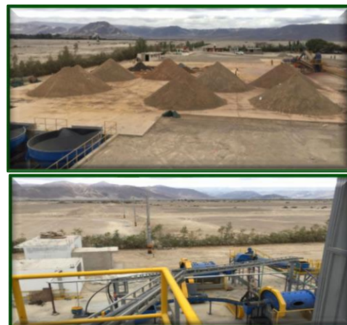
Figures 1 to 3: Vista Gold Plant – Leach Tanks for gold recovery (left), Crushed ore stockpiles ready for grinding and processing (upper right), and ball mill grinding circuit and conveyor feed to leach tanks (lower right)
