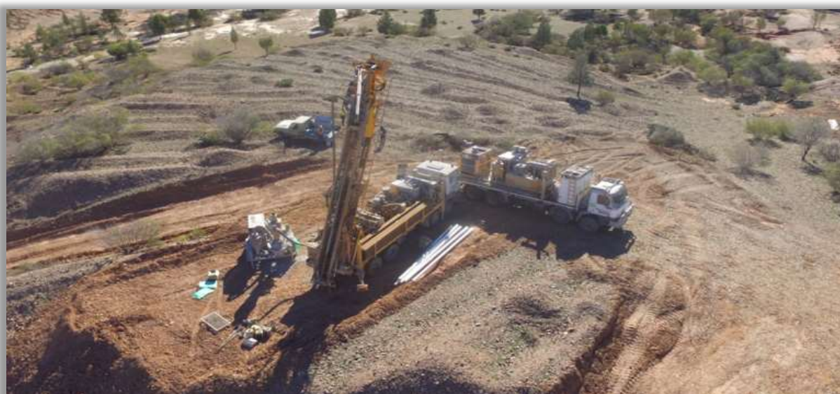
Figure 1: RC Drilling Rig at the Tallebung Tin Project, on the edge of the historic Tallebung open cut pit.
