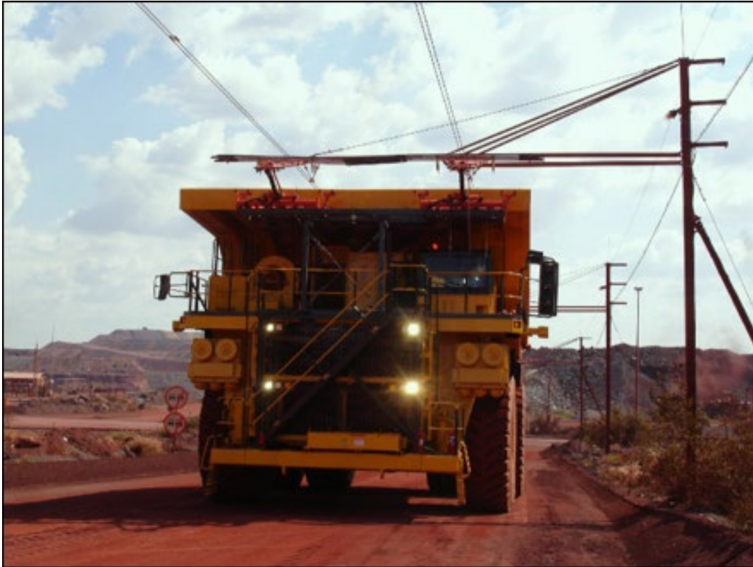
Figure 1: A trolley assist overhead transmission line for a haul truck. Photo supplied by Komatsu Australia.
