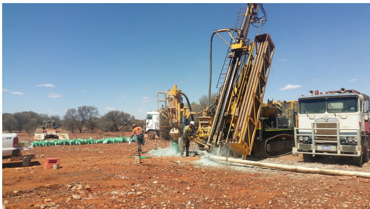
Photo 1: Larger RC rig commenced drilling of deeper hole to test potential depth extensions, Reedy South Gold Project
