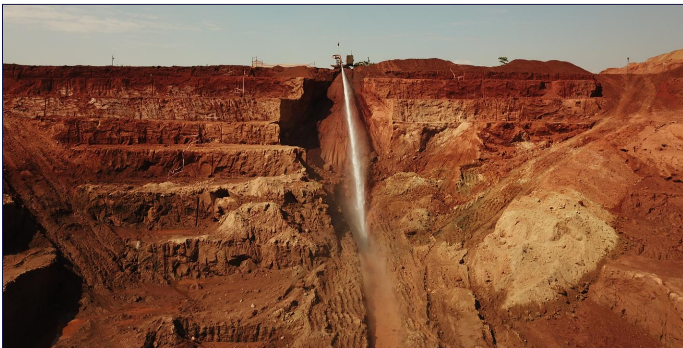
Figure 1: Hydraulic mining of Kasiya test pit
