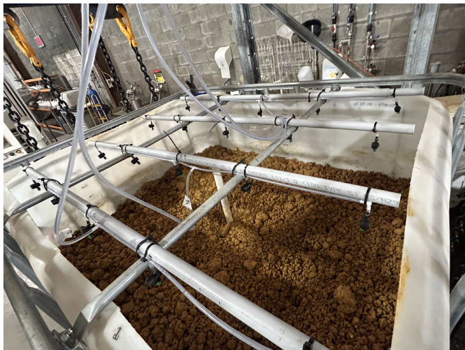
Figure 3: Bulk Leach with dripper system applying lixiviant for leaching
