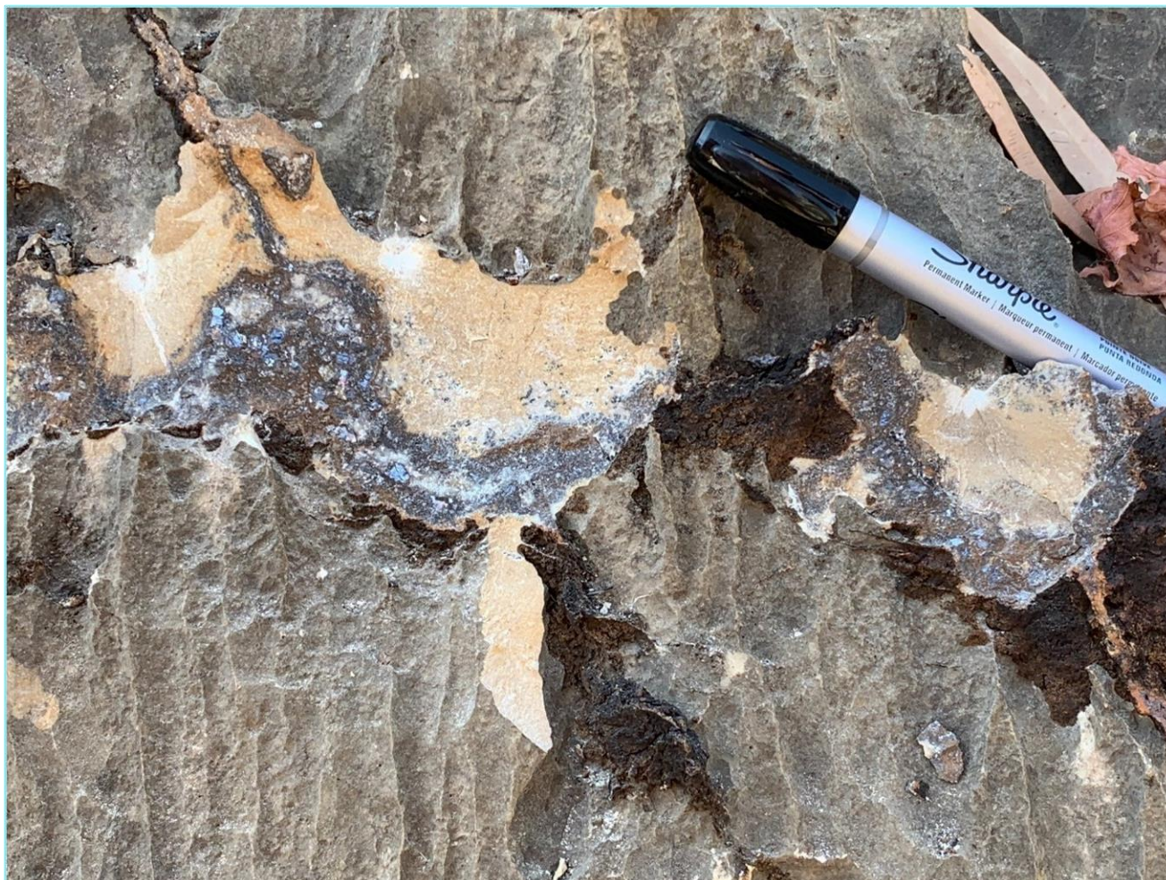
Figure 3: Visible galena and hydrozincite (after sphalerite) discovered 350m north of historical drillhole EPP11, near Devious gossan (808496.237mE, 7952741.769mN)
