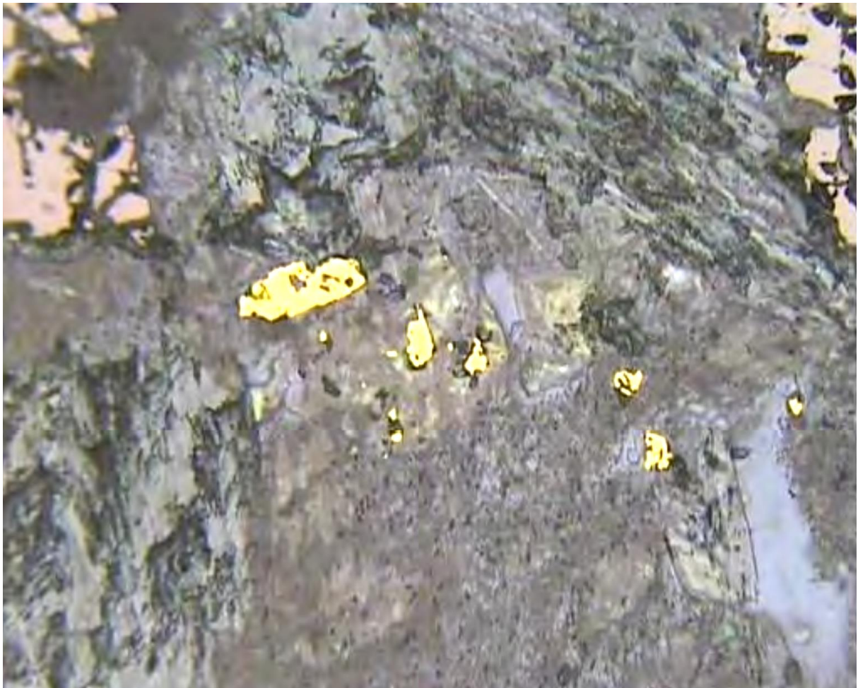
Figure 2: photomicrograph of sample 1370002.20 from 1,295.2 metres, showing fine grained chalcopyrite intergrown with secondary propylitic-style alteration minerals. Whilst only present in trace quantities, the importance of the intergrowth of chalcopyrite with distal porphyry-style late magmatic/hydrothermal stage alteration minerals is that it suggests that the parent intrusion (the source of these QDP dykes) is fertile (ie, enriched in metals, sulphur and water) and has produced a late stage metal and sulphur-rich fluid of the kind which can form copper and/or gold enriched zones.
