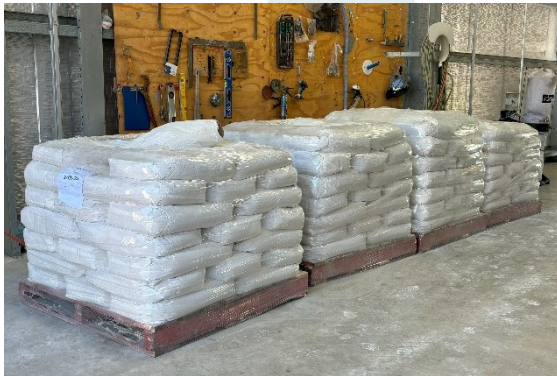
(left) four pallets of milled Toondoon kaolin ready for calcination and production of HRM
