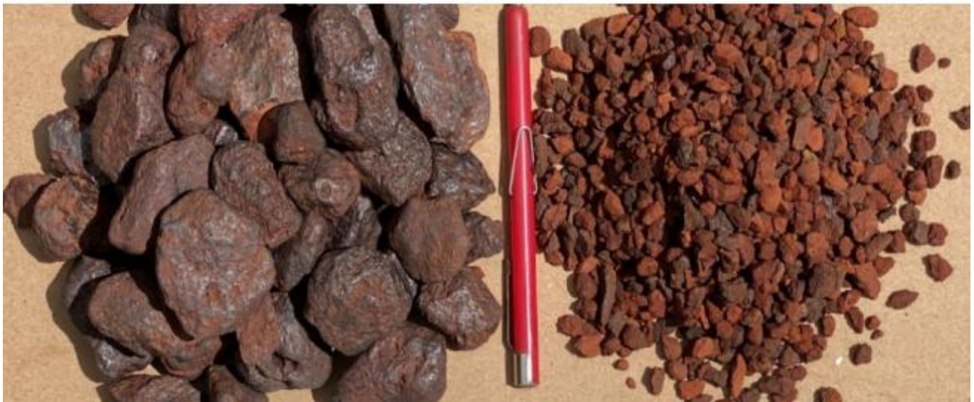
Figure 3. Bekisopa's DSO resource has the potential to produce a Lump product at an average 61.8% Fe grade (left) and a Fines product at an average 61.4% Fe (right), over the PFS LOM.
