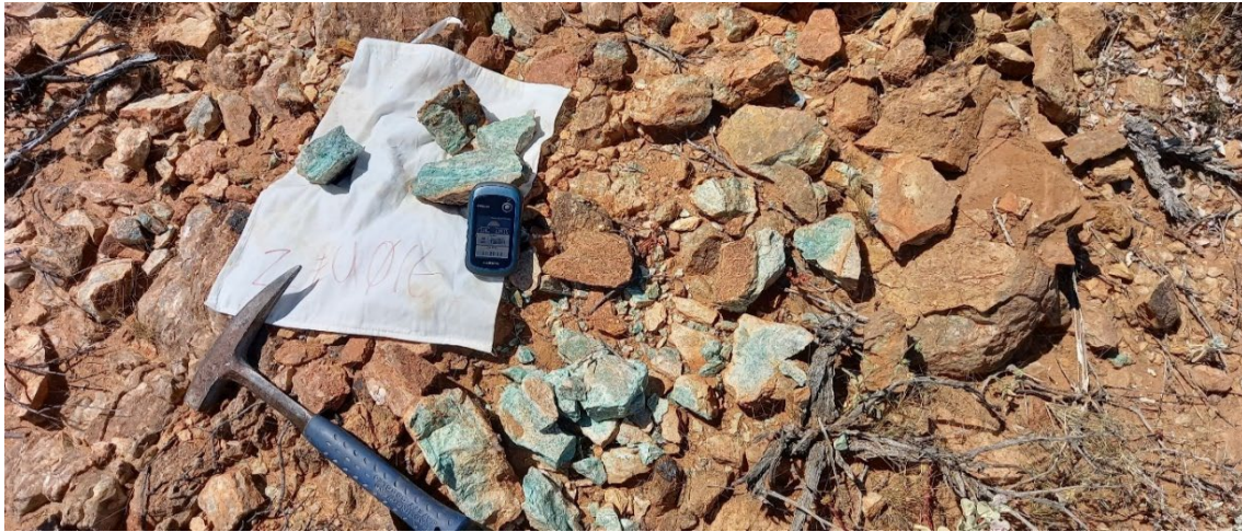
Figure 5. Detail of mineralised outcrop. (Sample# ZEU016 = 1.4% Cu, 0.19% Pb, 125 ppm Zn & 18.4 ppm Ag)
