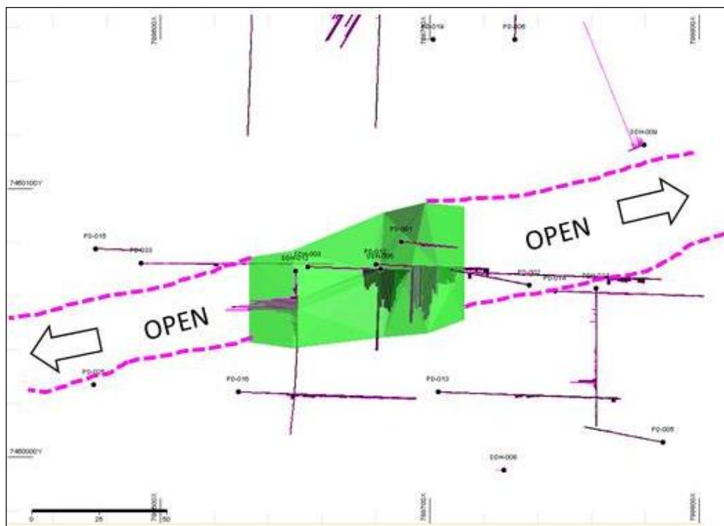
Figure 5: Plan of the Window Deposit (resource in green) drill hole traces and copper histogram plot – Showing Extension Targets
