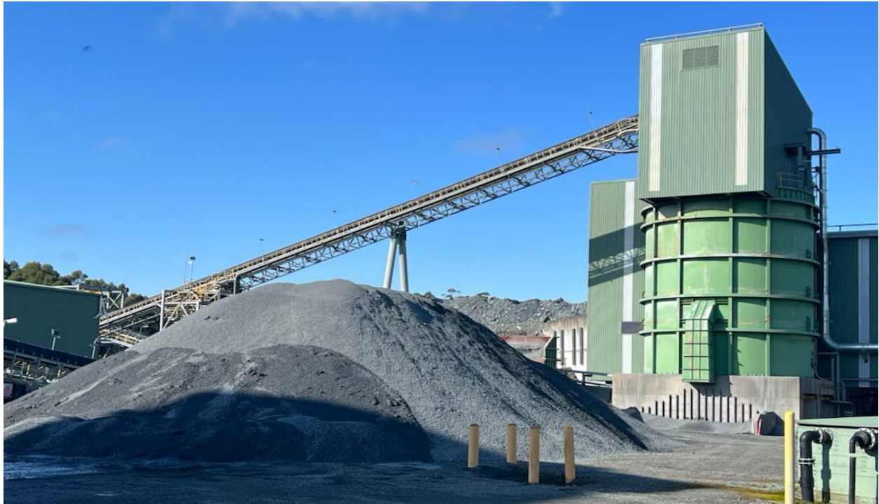
Figure 5. Stockpile of crushed ore adjacent to the fine ore bin from the crushing circuit.
