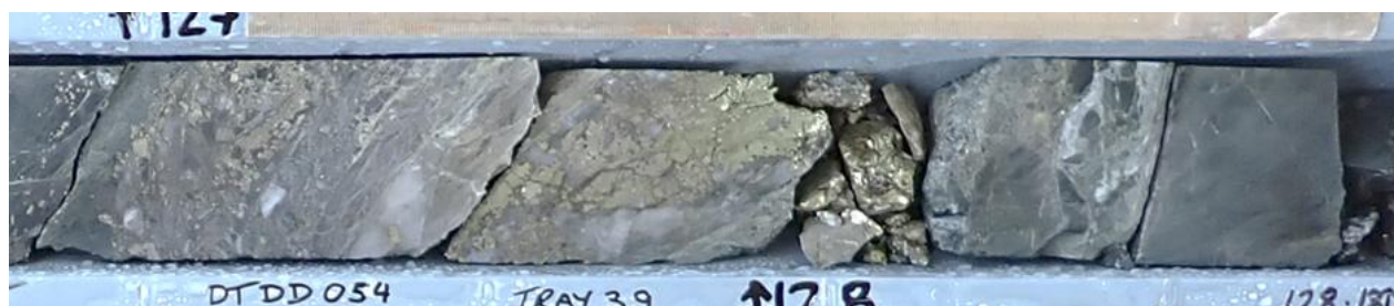
Figure 6 – Examples of the Mine Lode including quartz-pyrite-chalcopyrite veining in chlorite-sericite altered volcanic in DTDD054 (127.8 – 128.2m).
