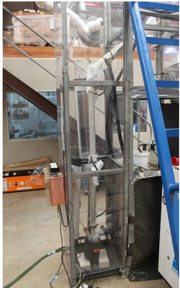
Image 4: Operational distillation column after commissioning
