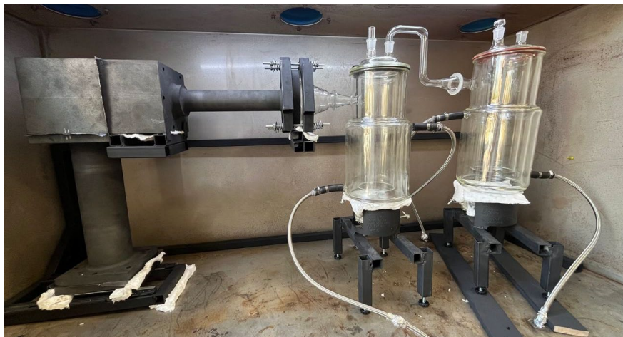
Image 1: Pilot extraction set up: graphite reactor and transfer tube
