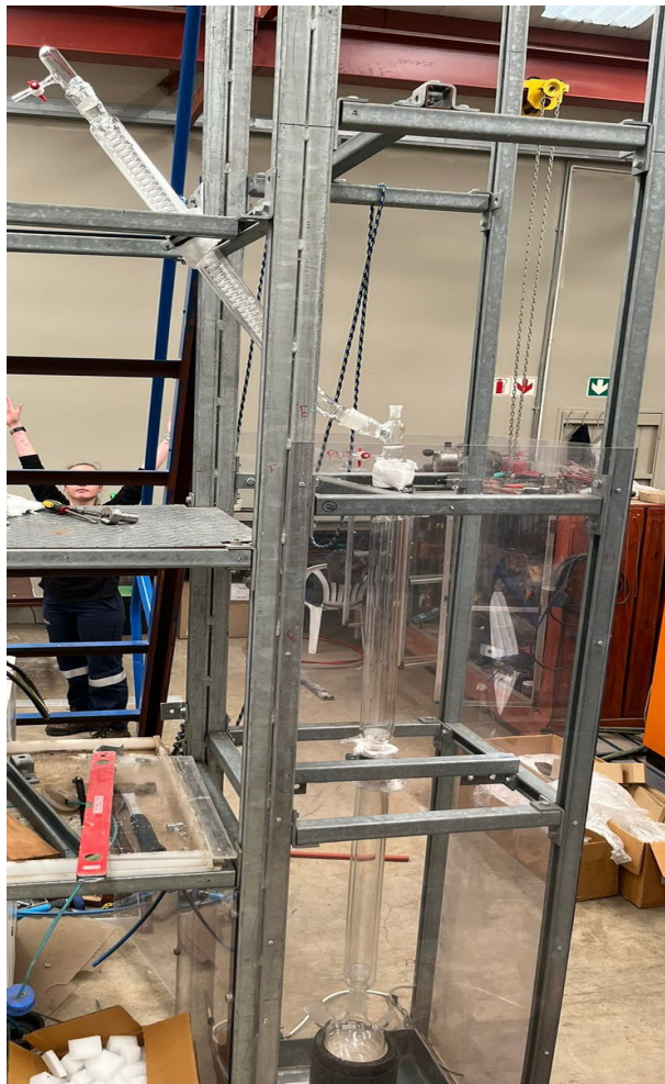
Image 3: Two-stage, 2" distillation column with thermal oil cooled condenser
