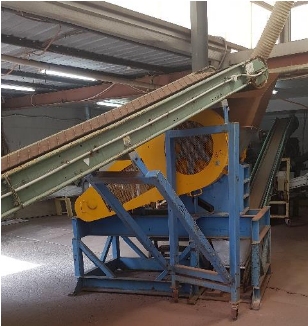
Plate 4 Feed hopper jaw crusher
