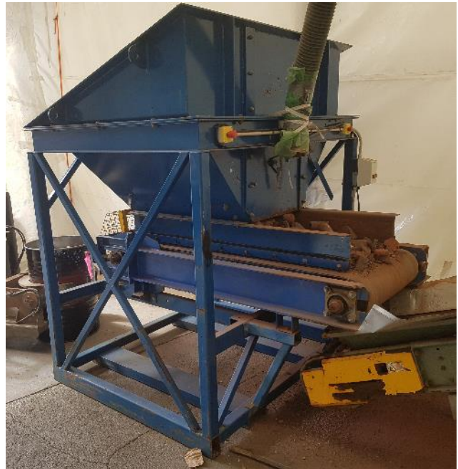
Plate 5 Trans hopper feed to prime crusher
