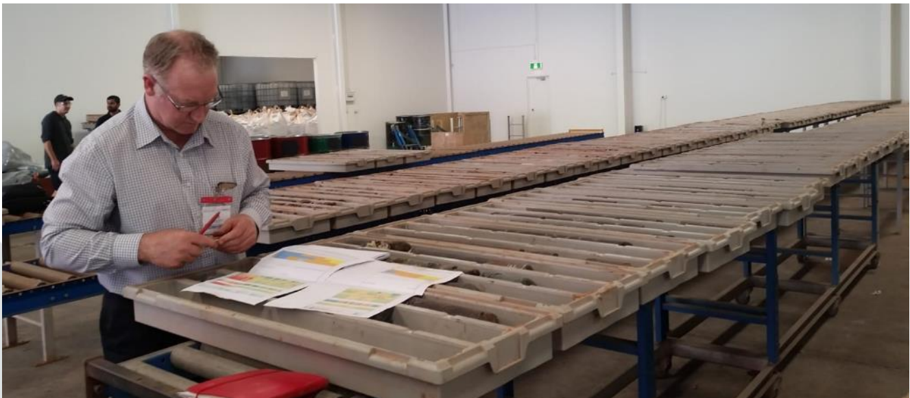
Plate 3 Bulk core sample test work preparation in the laboratory
