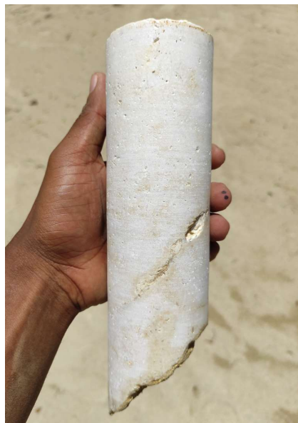
Fig 1 – High purity Soalara Limestone core
