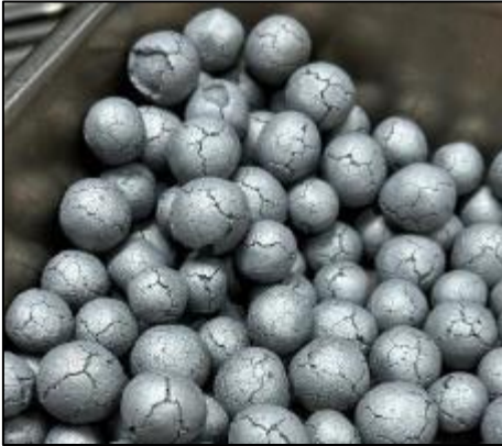
Metallised pellets after Linder test work
