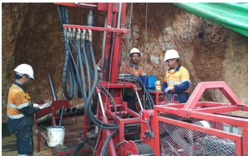
Figure 1. Man-portable rig drilling BWDD034 on Yegon Ridge.
