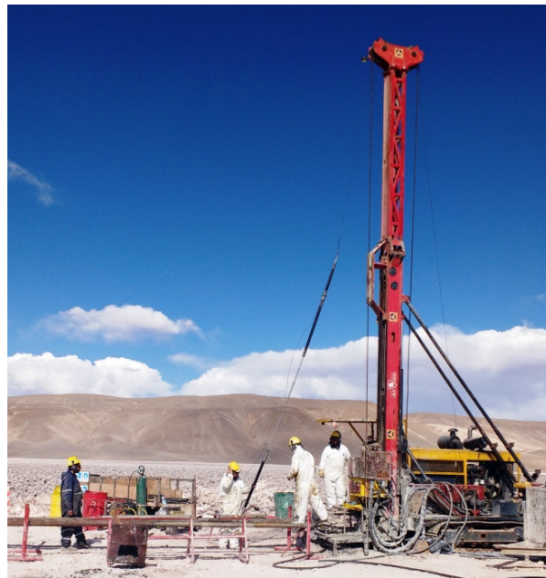
Photos 6 & 7. Rincon Lithium Project – Exploration diamond drilling operations
