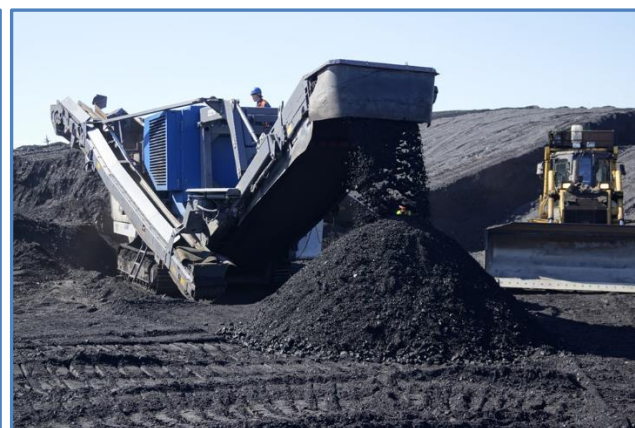
Coal crushing at the port stockpiles
