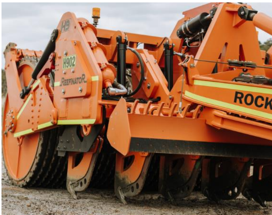
Figure 2 – The Rocksgone Dynamic Force Crusher (DFC) or Reefinator
