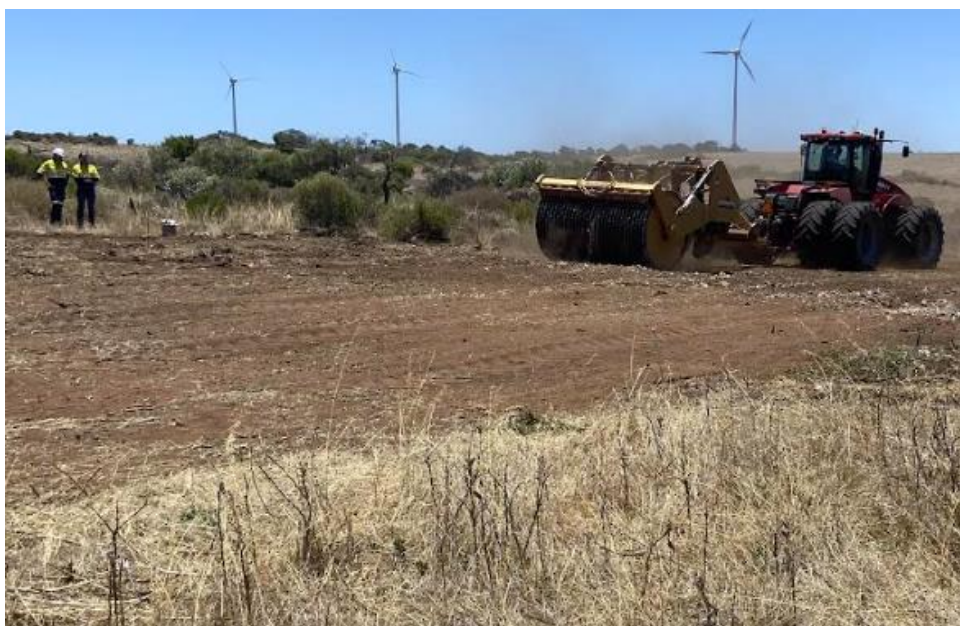
Figure 3 – The Rocksgone Dynamic Force Crusher (DFC) operating at the future Port Gregory mine site
